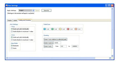
Figure 4 Plot Settings - Scaling and Zooming tab
